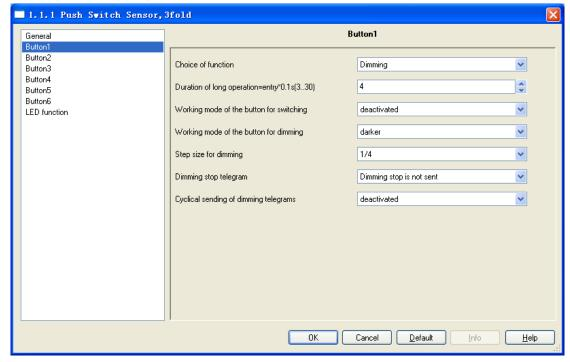
Fig.5.3 Parameter window "Dimming"
