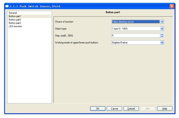
Fig.5.15 Parameter window "value dimming sensor"
