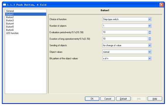
Fig.5.7 Parameter window "step-type switch"
