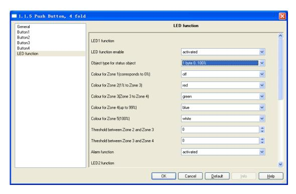
Fig.5.16 Parameter window "LED function" (1byte)
