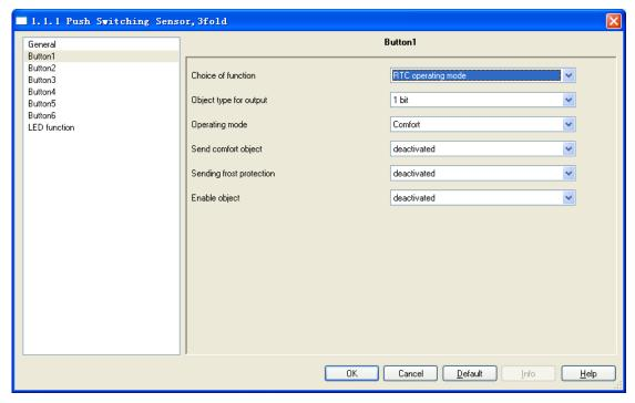
Fig. 5.9 Parameter window "RTC operation mode"
