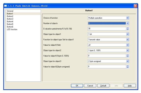
Fig.5.10 Parameter window "Multiple operation"
