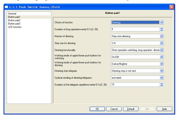
Fig.5.12 Parameter window "Dimming"
