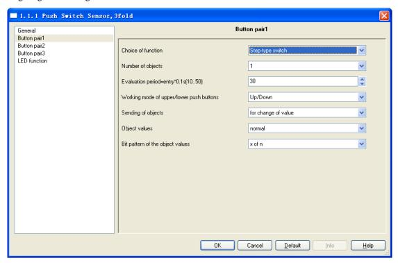
Fig.5.16 Parameter window "step-type switch"
